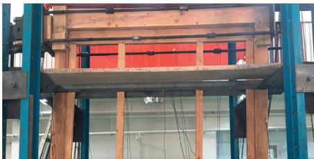
FIGURE 9: Loading fixture.
