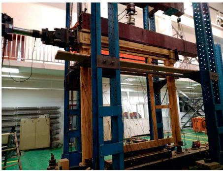
FIGURE 8: Vertical and horizontal loading devices.
