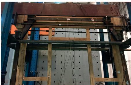
FIGURE 3: Channel steel and the diagonal brace.
